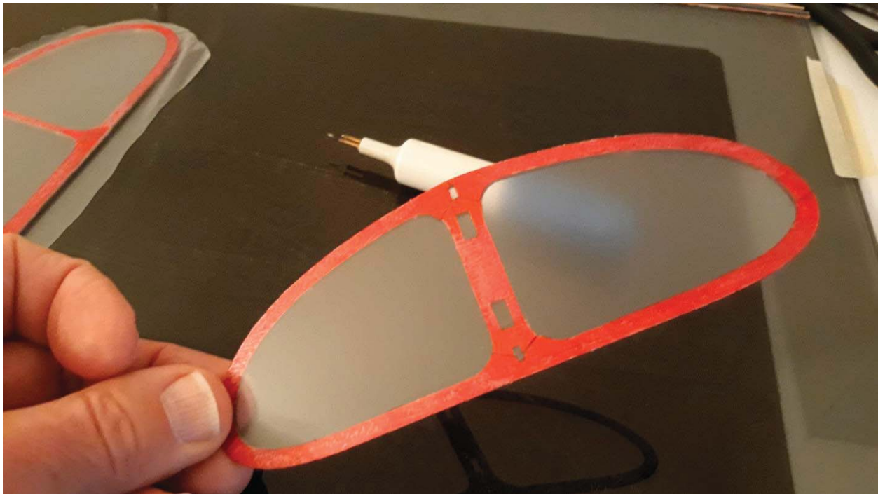
Excess produce bag material covering on the stabilizer has been trimmed with a surgeon's cautery.
