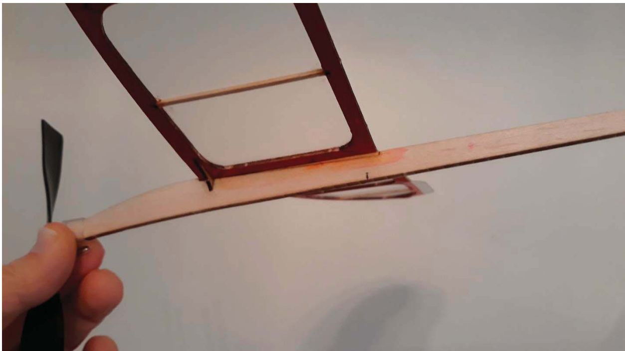
Note the 0.050" thick tapered shim glued between the wing and motor stick.
